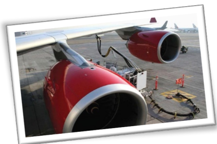
Ground refueling operations using Fuel Hydrant Delivery & Transmission Systems
